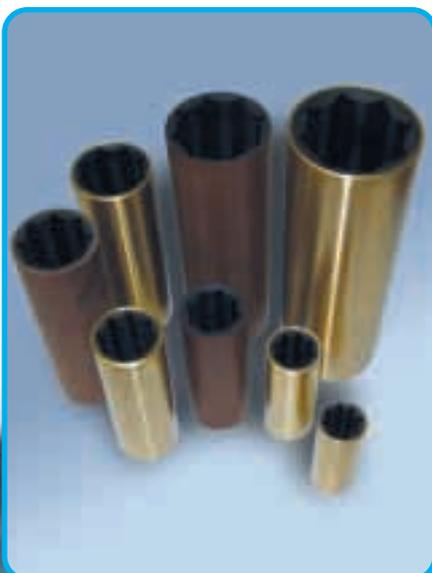
Aqualube water lubricated bearings have a shore hardness of  $70\pm 3$  and are suitable for operation in the temperature range of  $-25^{\circ}\text{C}$  to  $85^{\circ}\text{C}$ . Special compounds are available which will allow the working temperature to increase to  $200^{\circ}\text{C}$ . For temperatures above  $30^{\circ}\text{C}$  advice should be sought from the Technical Department relating to the clearance between bearing and shaft.
